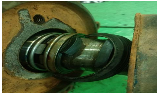
Gambar 3. Pecah nya mechanical seal
