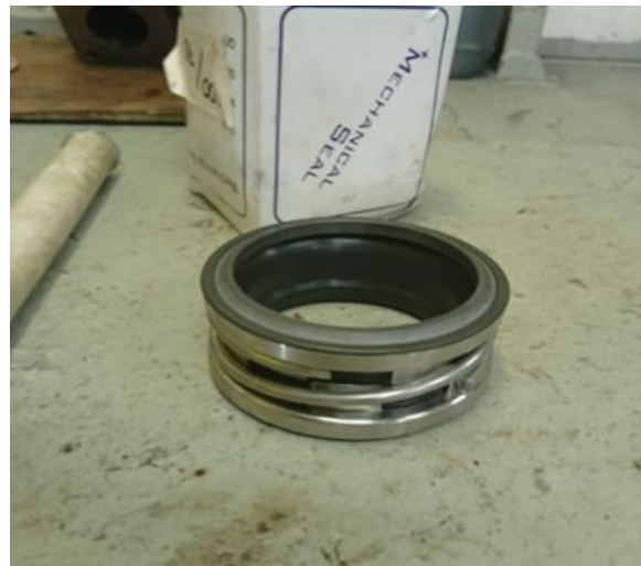
Gambar 4. Mechanical seal baru
