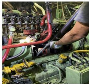
Gambar 3. Pelepasan Baut Connecting Rod.
