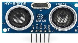
**Gambar 3. Sensor Ultrasonik HY-SRF05**
