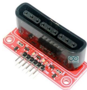
Gambar 3. Module Stick PS Wireless
