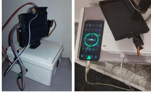
**Figure 7.** Physical prototype of the dual-axis tracker in a PVC enclosure (left), and a field demonstration of powering a mobile phone from stored energy (right)
