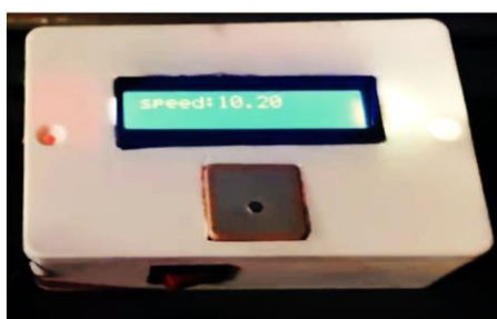
Figure 20: A plastic box includes two Arduino UNO boards, GPS, GSM modules and MPU-6050 sensor
