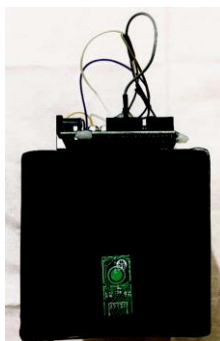
Figure 19: Back-view of rear radar system that faces the backward vehicles
