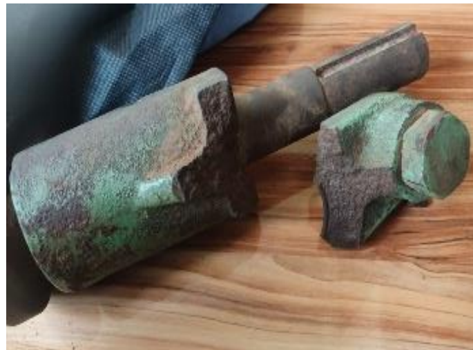
Figure 3. Example of a Broken Rubber Wheel Mount from the Previous Period.
