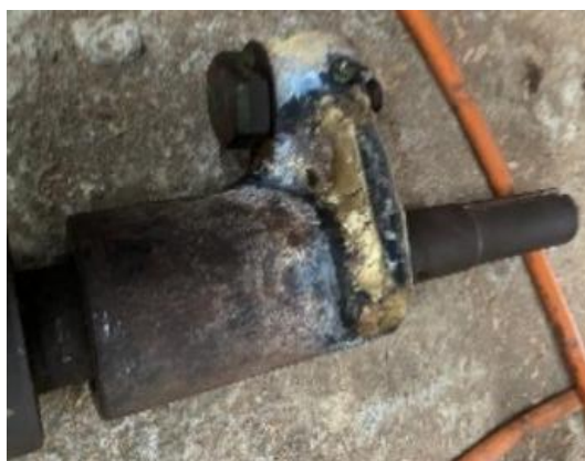
Figure 4. Example of Welded Rubber Wheel Mounting Results from the Previous Period.
