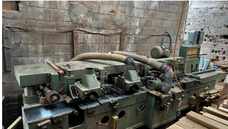
Figure 1. Wood Profiling Machine with 90 m/hour Capacity.
