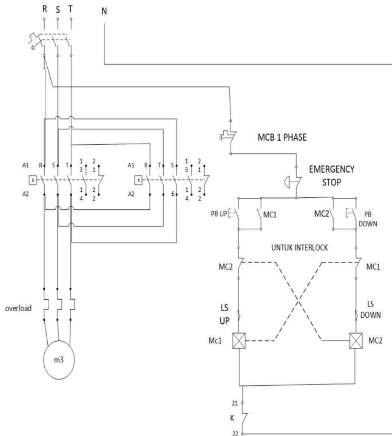
**Gambar 3.** Wiring Diagram
