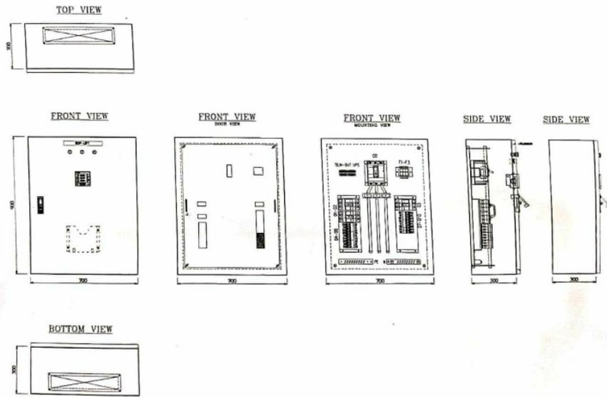
**Gambar 1.** Layout Panel Listrik Lift
