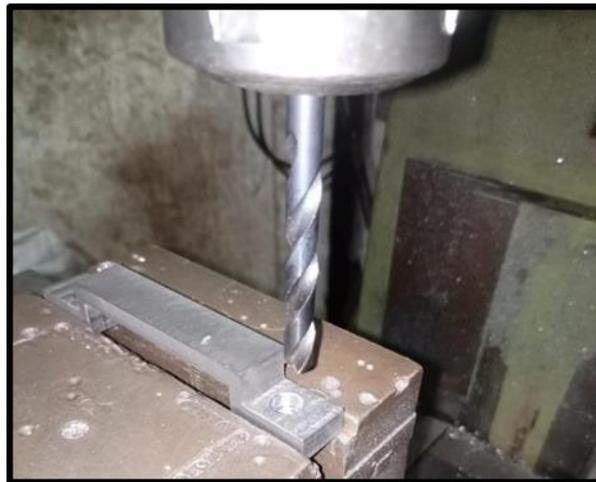
**Gambar 7. Proses *Drilling* Mata bor 10mm**
