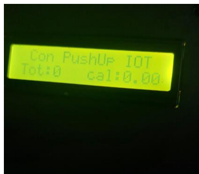
Gambar 4. Tampilan LCD I2C
